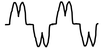
Typical current through LPF output stage
