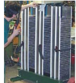
Partially assembled reactor with PolyGap™ core
