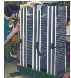
Partially assembled reactor with PolyGap™ core
