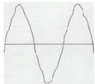
Input current waveform (6-pulse rectifier with APQ Low Pass Harmonic Filter)
