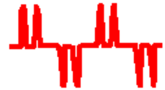
Input current waveform (6-pulse rectifier)
